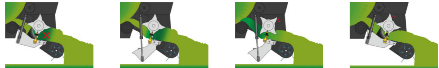
In the event of a blockage, the rear part of the cutting floor is lowered by 500 mm.
