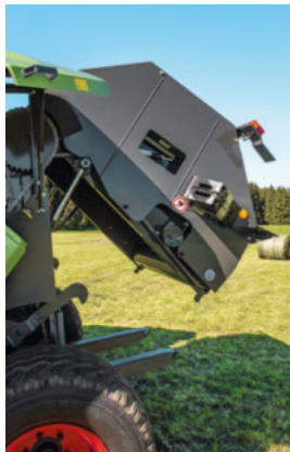
A pin on the tailgate ensures that it can be reliably closed even when used on slopes.
