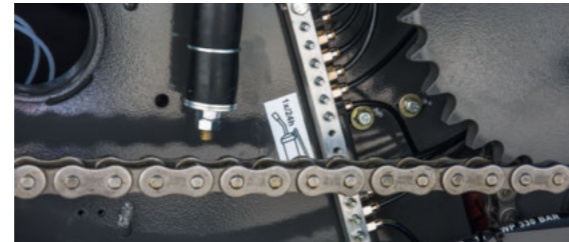
■ The quantity of oil to be used to lubricate the tracks is individually adjustable.
